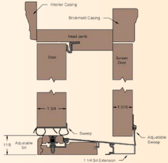
Non-Impact Prehang Details with Standard Jamb and Inswing Sill and Storm Door Attached
